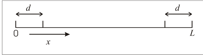
Figure 4.2: One-dimensional calculation window. PML's are located in the layers of thickness d on the left-hand and right-hand side of the window.
